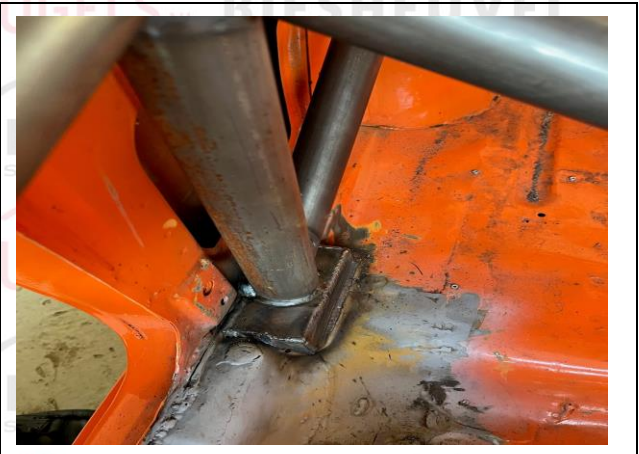
PHOTO 4 MAIN ROLLBAR TO FLOOR ATTACHMENT
